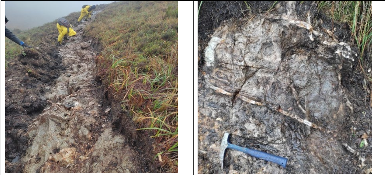
Figures 7 and 8: Porphyry with intense quartz stockwork with pyrite and traces of chalcopyrite
